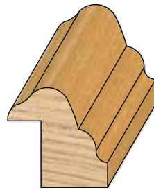
PROFILE # DIMENSION 2424PR 3/4" \times 3/4" * 1/4" \times 1/2" RABBET.
