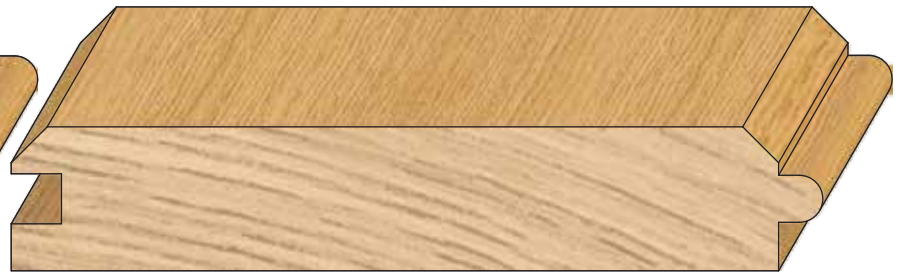
PROFILE # DIMENSION 24128TVG \frac{3}{4}'' \times 4'' (FACE)
